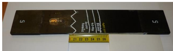
Figure 20: Crack propagation for tension load
