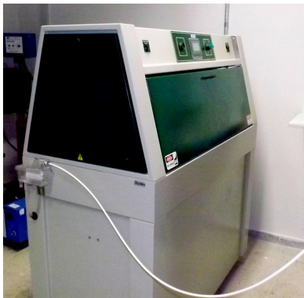
Figure 1: Aging chamber used for accelerated aging studies.
