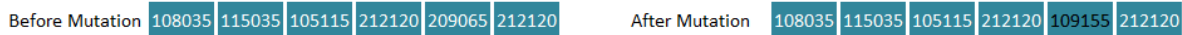
Figure 7: mutation for a six layers laminate in position 5 and applying of both methods
