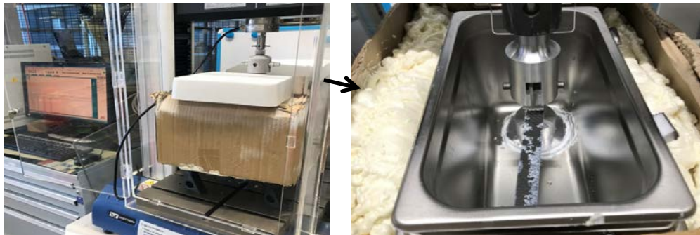
Figure 3. The cryogenic test setup for DCB testing.
