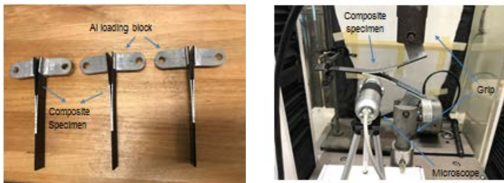
Figure 2. Composite DCB specimens attached with loading blocks and the loading blocks gripped through pins with the Instron tensile tester.
