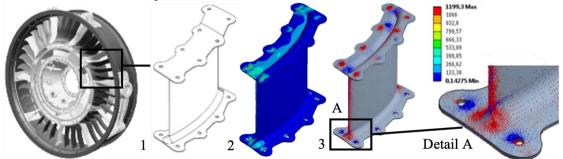
Figure 5: Concept for structural vane with double-T-shape (1), associated stress peaks (2) and main principal stresses for design of fibre architecture (3)
