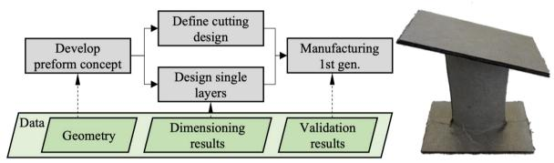
Figure 8: TFP-manufactured preform for a structural vane with its design process
