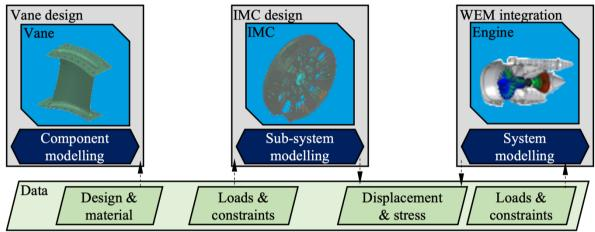
Figure 6: Modelling scales of the structural vane with different associated models, methods, input and output data
