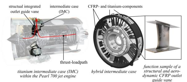
Figure 1: Rolls-Royce Pearl 700 (left) with function-integrated IMC, composite-metal IMC of future jet engine generations (centre) and function sample of a CFRP outlet guide vane (right) [8]
