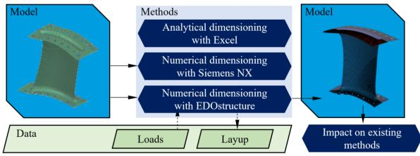
Figure 7: FE-Model of structural vane as part of dimensioning process step with different associated methods, input and output data
