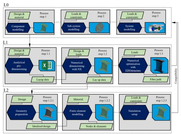
Figure 10: MMD process step diagram for a section of the vane development
