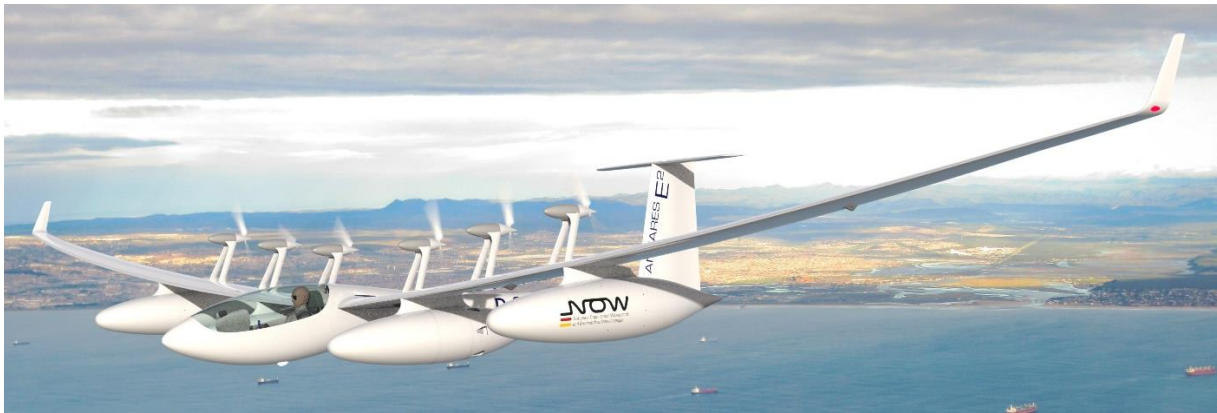
Figure 2: Aircraft with aerodynamic underwing pods as an attractive option for H_2 -storage [6]
