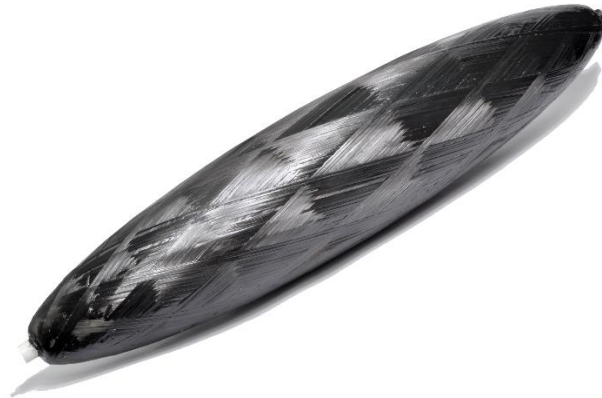
Figure 12: First filament wound layer of the ellipsoid pressure vessel
