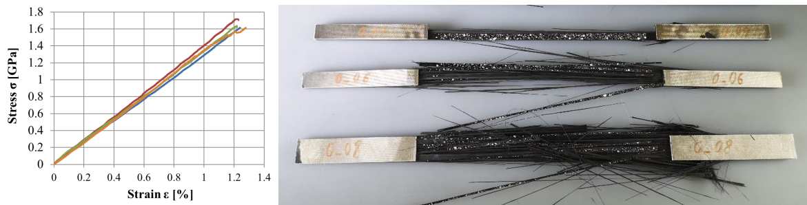
Figure 6: Tensile test stress-strain-curves of 0°-UD-CFRP-specimens made of HTS40 fiber and L20 resin system (modified according to [9], left) and their typical failure mode (right)
